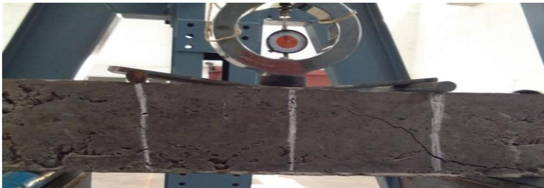
Figure6 Cracking of Specimens in loading frame
