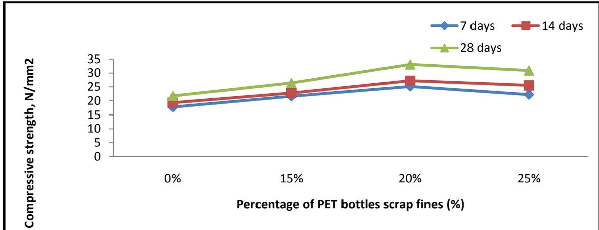
Figure 5 Compressive strength vs PET bottles scrap fines (%)
